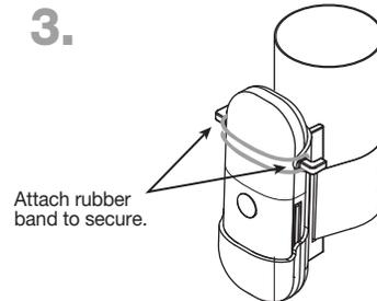
Attach rubber band to secure.
