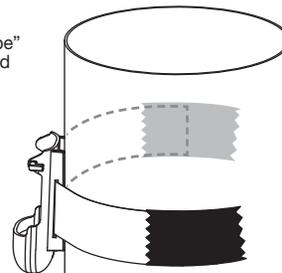
For large body tubes, use 2 pieces of "electrical tape" to secure strap to body tube.
