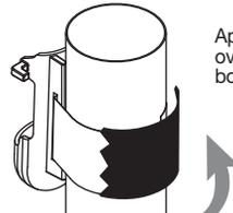
Apply "electrical tape" over paper strap and body tube.
