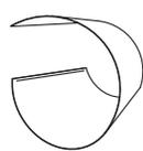
3. Apply glue to one edge of wrap and apply joiner, centered over edge as shown below. Leave equal space between the front and back of joiner.
