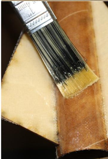
**STEP 4** IF Mylar was used on the fins, remove. Apply external fillets where each fin meets the airframe. Apply each set and allow to cure before moving onto the next.
