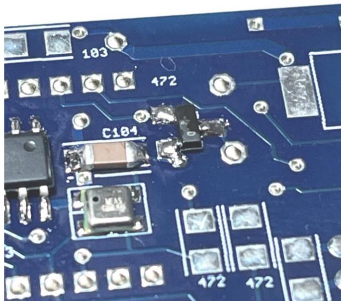
— Mount the three 4.7K resistors (marked “472”)
