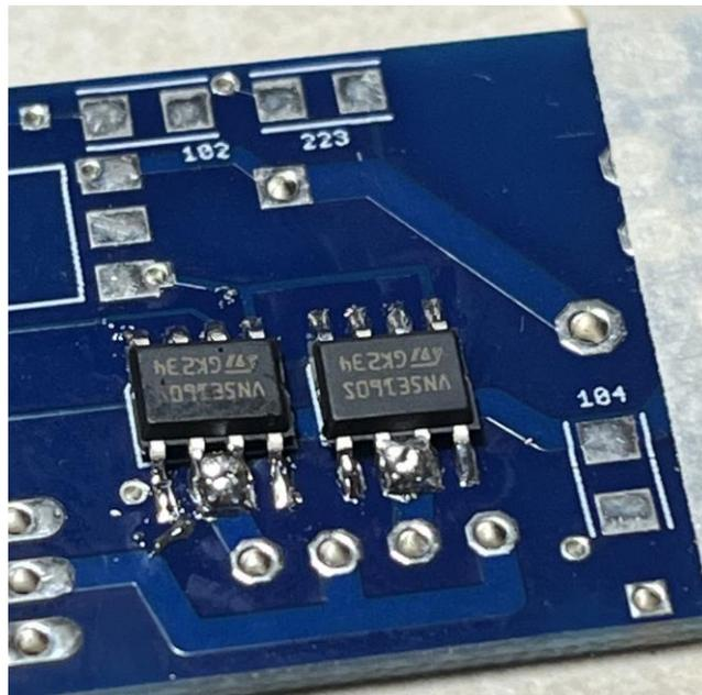
— Mount the 100K resistor (marked “104”)
