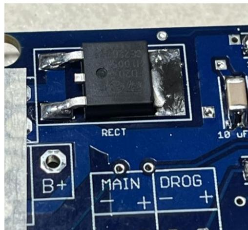
That completes the mounting of the SMT parts on the top of the board. Remove the tape and toothpicks from the board.
