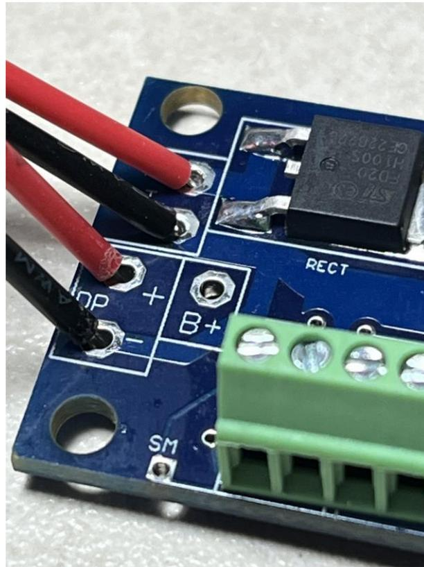
In the picture above, the two power leads on the BAT pads are powering the Quantum's flight computer, and the two power leads on the "DP" pads are powering the deployment outputs.
