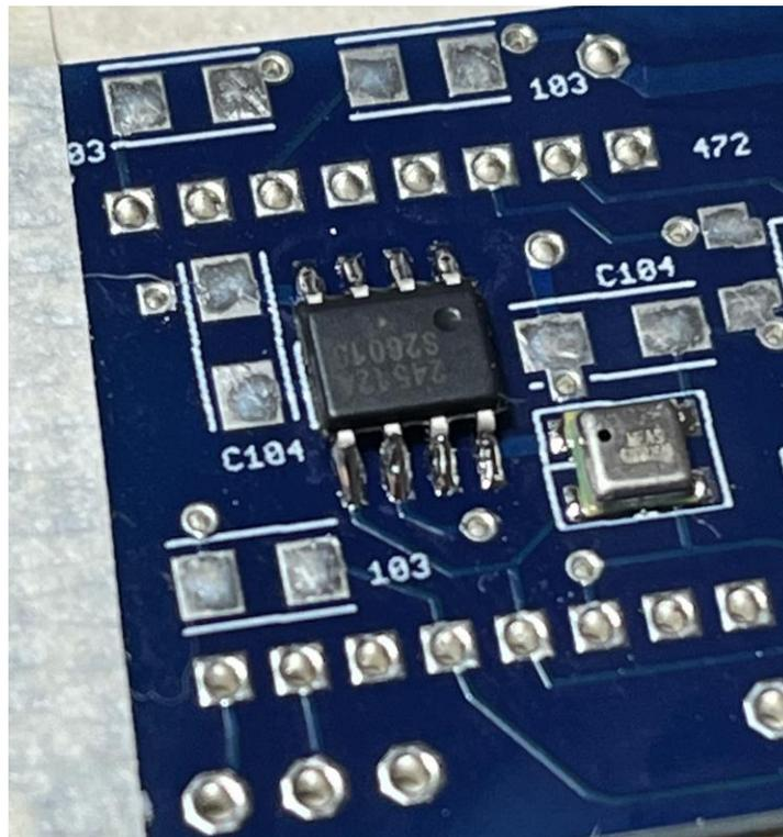
— Mount the 10K resistor (marked “103”)
