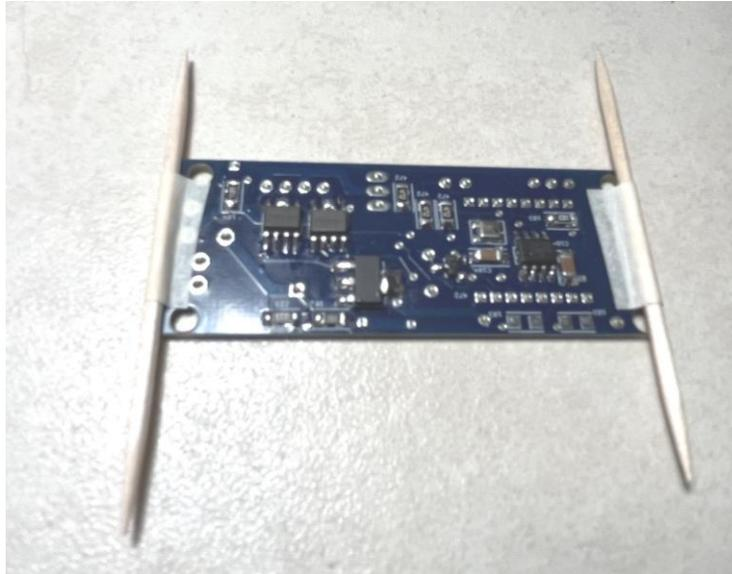
Now, turn the board over and lay it down. The toothpicks should stand the board off from your work surface about 1/8”... this protects the sensitive baro pressure sensor and the other previously bottom-mounted components while you’re working on the top of the board.
