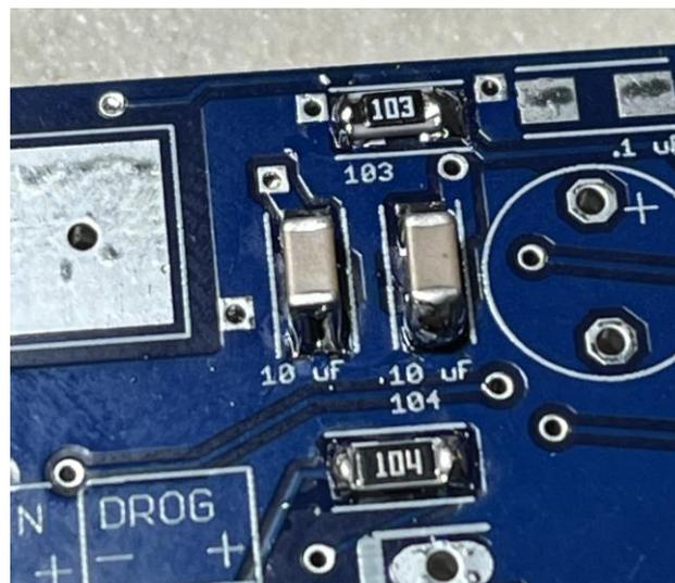
— Mount the 0.1 uF capacitor (unmarked brown part in PAPER tape)
