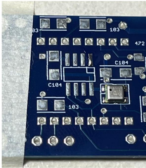
With tweezers, hold the EEPROM in place, and heat the lead over the tinned pad until the solder melts. Keep the heat on for another 3-4 seconds, then remove the iron and let the pad cool.
