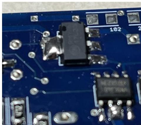
— Mount the 1K resistor (marked “102”)
