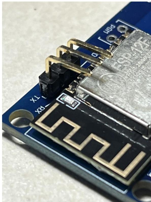
— Mount the 3V3 header pin (Optional – for use with the Eggtimer Telemetry Module)
