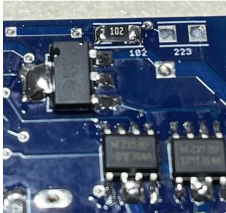
— Mount the 22K resistor (marked “223”)
