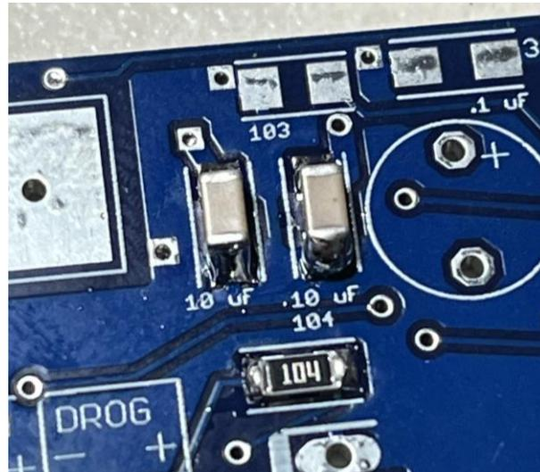
— Mount the 10K resistor (marked "103")
