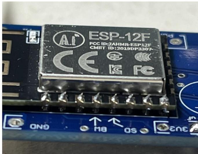
Now, turn the board over so the WiFi module is on the bottom, and solder the leads to the boards. Again, use only enough solder to ensure that you have a good mechanical connection. Clip the leads as you go, making sure that the remnants don't land somewhere on the board.
