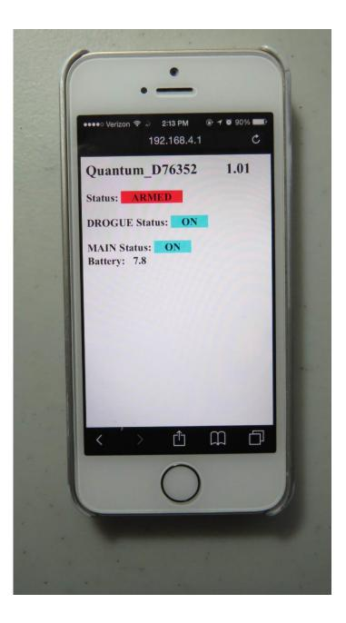
This page looks a lot like the status page, but the status is changed to "ARMED", it doesn't initially have the validation code/box, and only the channel continuity status and the battery voltage are displayed. A few seconds later you should start hearing the buzzer beep about once per second. This is an audible confirmation that the Quantum is now in flight sequence mode, and you're ready for launch.
