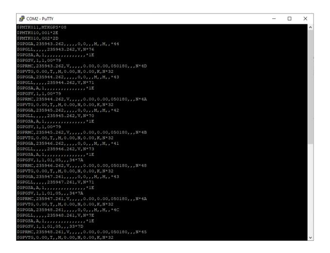
If you see this, then congratulations... the GPS is working, and you can go on to mounting the RF module. Disconnect the battery, the cable, and remove the jumper on the RUN pins... you'll put it back later after you mount the RF module.
