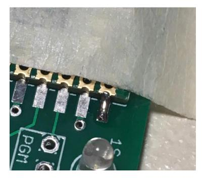
Inspect the pad that you just soldered with a 10x jeweler's loupe, there should be a nice fillet of solder between the "half-moon" pad on the RF module and the pad on the PC board.
