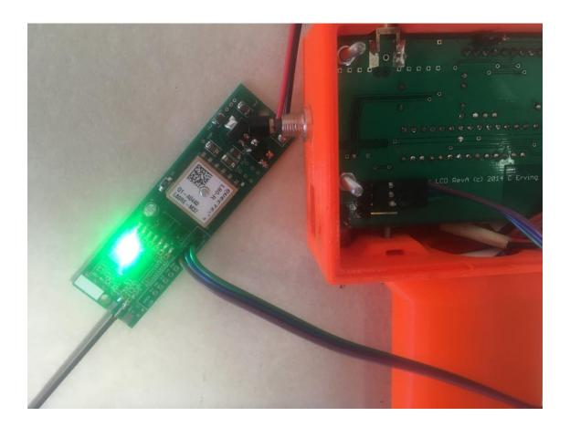
• Turn on the LCD receiver's power... the TX should also come on with BOTH the RED and GREEN LED's on the RF module lighting up. If it does NOT come on like this, immediately turn off the LCD's power and check your connections.
