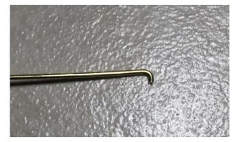
\_\_\_\_\_ Put the bent end of the antenna into the hole on the top of the board marked ANT, but **do not** solder it in. Tape it down so that it points straight out from the board
