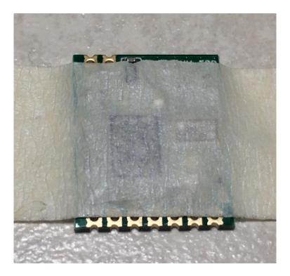
\_\_\_\_ Carefully position the Hope RF module on the board so that its pads line up in the center of the top pads, the "half-moon" cutouts on the module should be centered on the pads on the board. Using the tape on the RF module, secure it in position.
