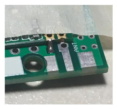
\_\_\_\_\_ DO NOT solder the pad marked "ANT" at this time... you'll solder it when you mount either the wire antenna or the RP-SMA connector. Leave the tape over the RF module for now, too.
