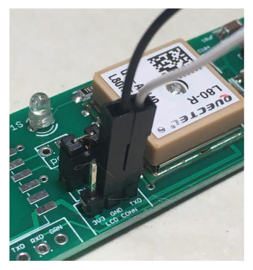
Plug the USB-Serial cable into your computer, and start the terminal program... the settings should be 9600 baud, 8 bits, no stop bits.
