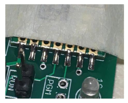
\_\_\_\_\_ Turn the board around, and solder the pad that is NOT marked "ANT". Inspect the solder joint carefully with a 10x jeweler's loupe, there should be a nice fillet of solder between the "half-moon" pads on the RF module and the pads on the PC board.
