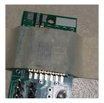
\_\_\_\_\_ Double-check the alignment. The "half-moon" cutouts on the end of the RF module pads should be squarely on the center of the PC board pads, on both ends of the RF module. If they are not, remove the module and reposition it until they are.
