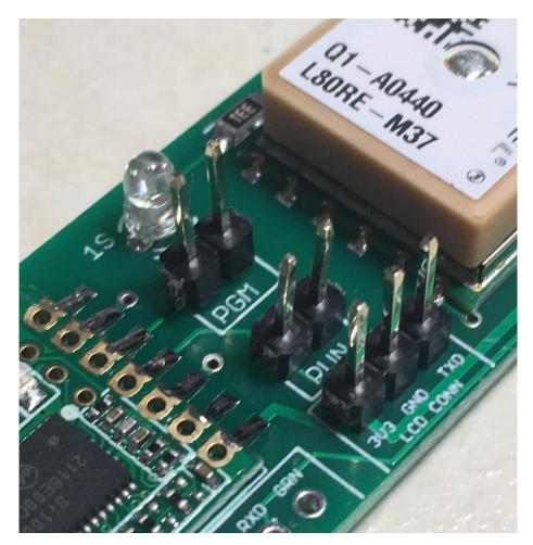
\_\_\_\_ Place the jumper on the RUN pads
