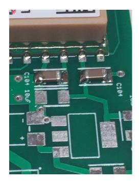
\_\_\_\_ Mount the 10 uF capacitor
