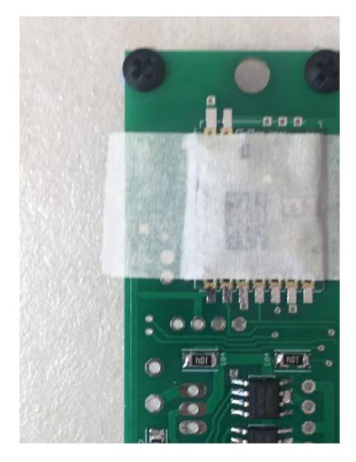
\_\_\_\_\_\_Solder the second pad from the bottom-right of the Hope RF module to the board. Make sure that the board is properly positioned after you solder this joint; if it moves, heat up the solder joint and move the board slightly so that it is properly positioned. Wait 30 seconds after soldering before continuing.
