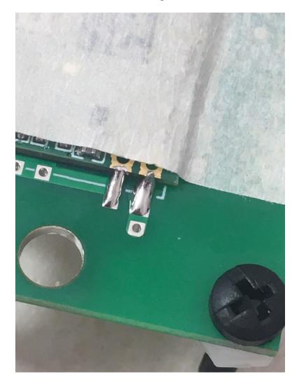
\_\_\_\_\_ Inspect all the solder joints on the bottom of the board, using a 10x jeweler's loupe. They should all be nice and shiny, and the solder joints should clearly bridge the parts with the PC board pads. If you have any questionable joints, we recommend that you remove any excess solder with desoldering wick, and resolder.
