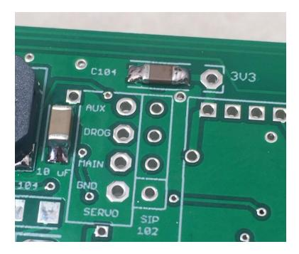
Mount the 100K resistor (marked "104")
