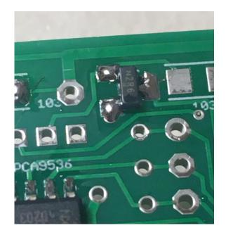
Mount the 10K resistor (marked "103")
