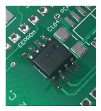
Locate the spot for the .1 uF capacitor right next to the EEPROM, it will be marked "C104" on the board. Solder in place.
