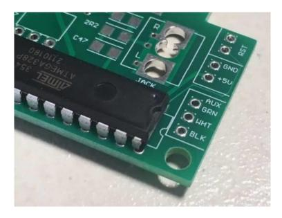
Turn the board over. Solder ONLY two opposite corner pins, then turn the board upright again, and make sure that 1) you have the chip pointed in the right direction, and 2) the chip is seated completely against the circuit board. If you made a mistake, you will have to carefully unsolder the chip and fix the problem; two solder joints are a lot easier to fix then 28.
