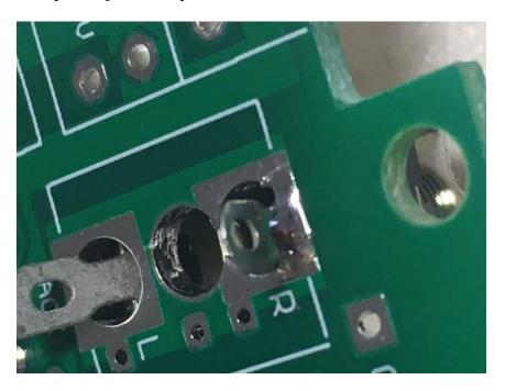
When you're satisfied with the alignment of the jack, generously solder the tabs to the outside edge of the pads... be generouts, but don't put so much solder that it starts running down the inside edge of the tabs, though, because you don't want any solder get into the jack itself. When you're done, clip the excess leads.
