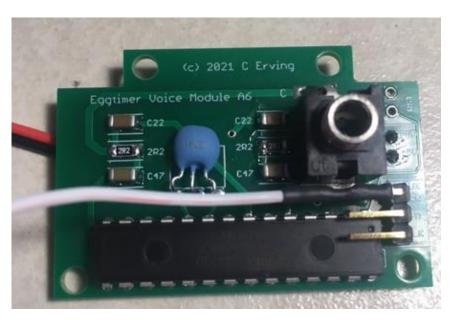
This completes the construction of your Eggfinder Voice Module board. Now, it's time to attach it to your Eggfinder LCD receiver board, and mount it in your case...
