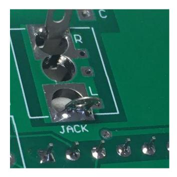
Take the 1/8W resistor, and slide it through the hole in the end tab, and gently guide it into the pad marked "C". Solder the wire to the "C" pad, then clip the excess wire on the other side of the board. Bend the tab down so that it's nearly flush with the jack, then solder the wire to the tab. Clip off the remainder of the resistor.
