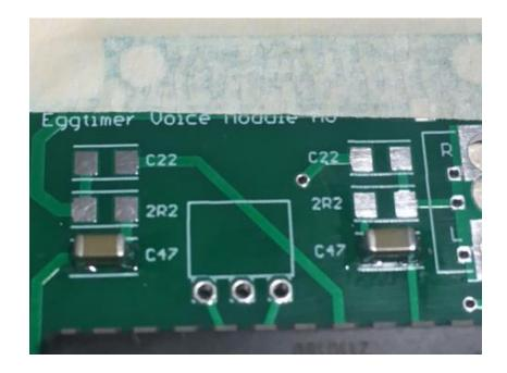
Locate the spot for the two 2.2 ohm resistors, just above the two 47 uF capacitors that you just mounted. Solder in place.
