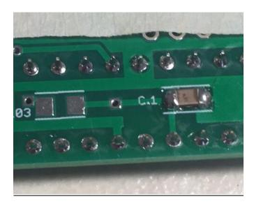
Turn over the board so that it's on the "bottom" side, where the processor solder joints are. Locate the 10K resistor on the board, it's in between the row of soldered pins. Solder in place.
