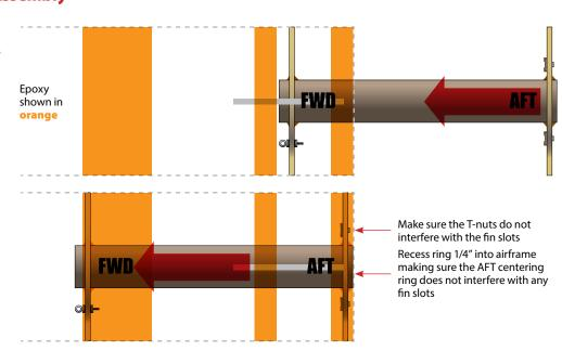
You may always add more epoxy to the FWD ring by drizzling epoxy onto the ring from the FWD end of the booster.
