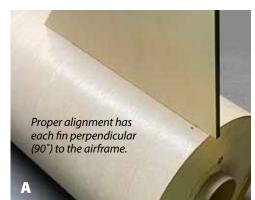
repeat the epoxy process. Repeat with the last remaining fin.
