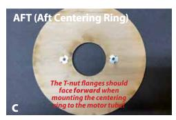
**C**. Press the T-nuts into the laser cut holes in the AFT centering ring. The flange side of the T-nuts will be **forward** when mounted on the motor tube.
