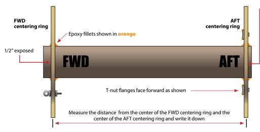
**A**. Epoxy the FWD centering ring onto the motor tube leaving 1/2" of the motor tube exposed. Make sure the eye bolt faces forward as shown.
