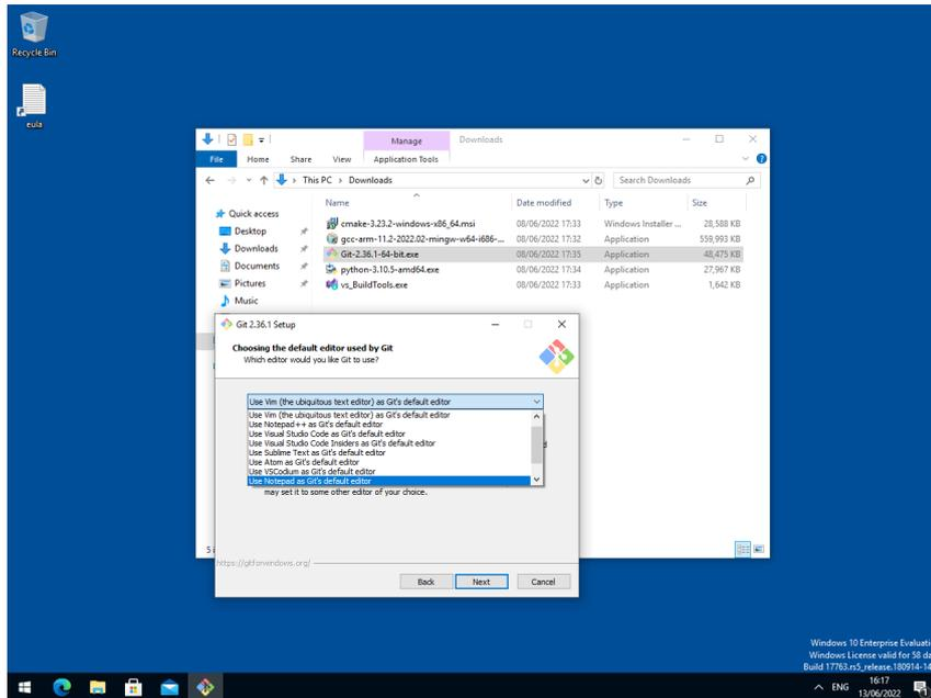
Ensure you tick the checkbox to allow Git to be used from 3rd-party software and, unless you have a strong reason otherwise, when installing Git you should also check the box "Checkout as is, commit as-is", select "Use Windows' default console window", and "Enable experimental support for pseudo consoles" during the installation process.
