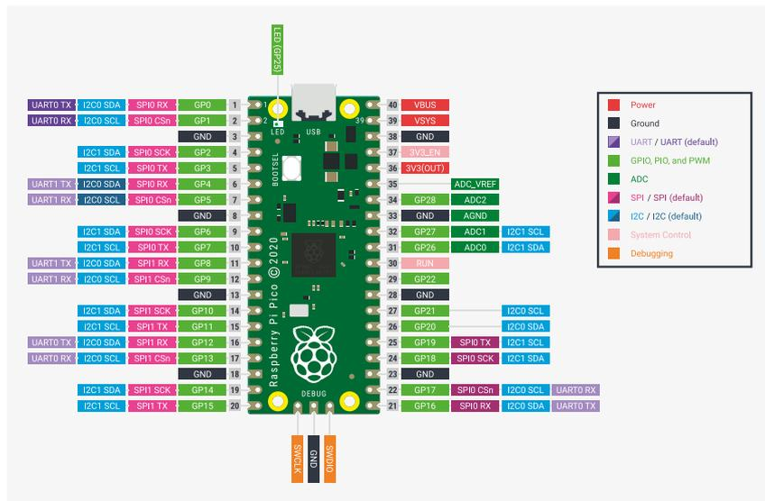
On a Raspberry Pi, you can connect the Pi GPIOs directly to Pico's SWD port, and load code from there. On other machines you will need an extra piece of hardware – a *debug probe* – to bridge a connection on your host machine (like a USB port) to the SWD pins on the Pico. One of the cheapest ways to do this is to use *another* Pico as the debug probe, and this is covered in [Appendix A](#).
