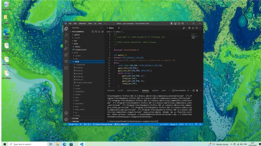
To build one of the examples, click the "CMake" button on the sidebar. You should be presented with a tree view of the example projects; expand the project you'd like to build, and click the small build icon to the right of the target name to build that specific project.
