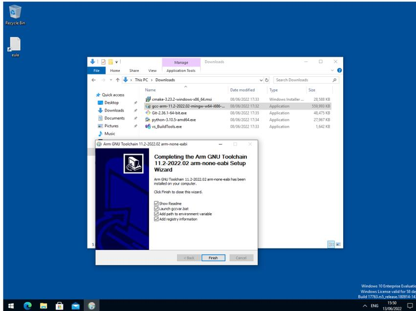
During installation you should tick the box to register the path to the Arm compiler as an environment variable in the Windows shell when prompted to do so.
