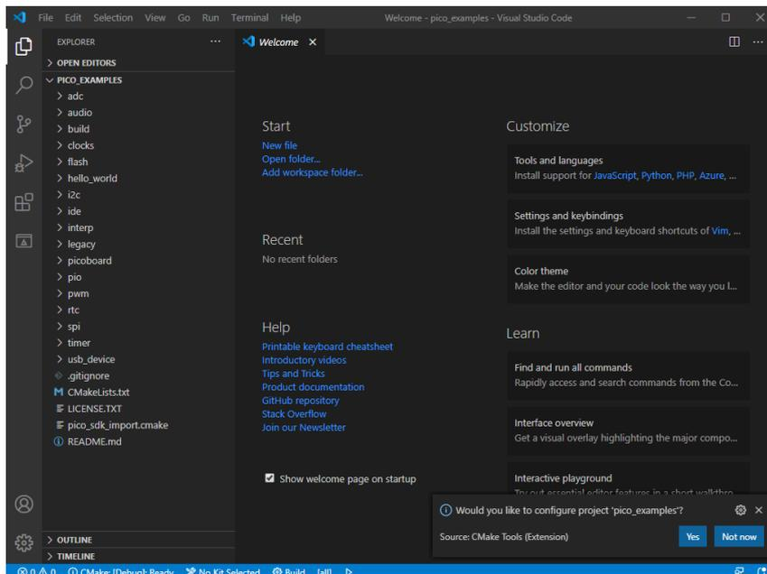
Go ahead and click on the "Build" button (with a cog wheel) in the blue bottom bar of the window. This will create the build directory and run CMake and build the examples project, including "Hello World".
