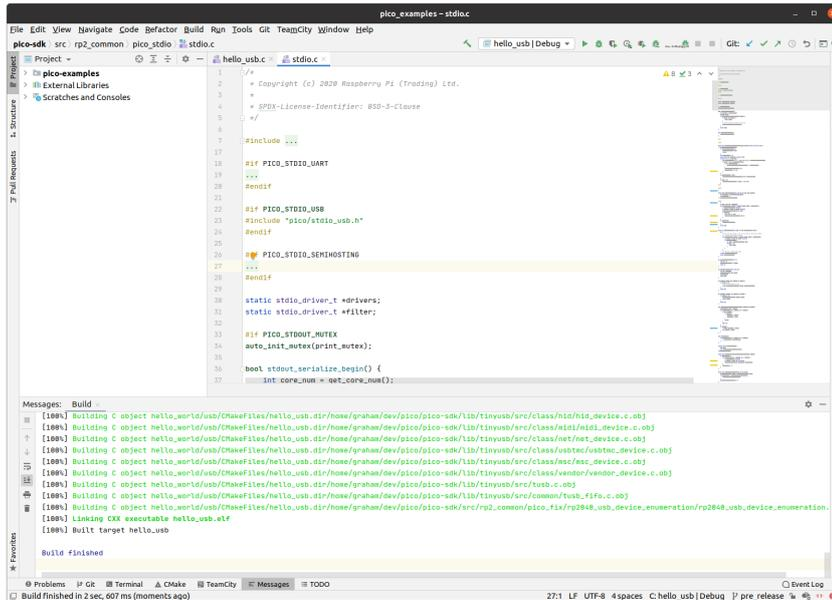
Note that the drop down selector lets you choose both the target you want to build and a CMake profile to use (in this case one of `Debug` or `Release`)
