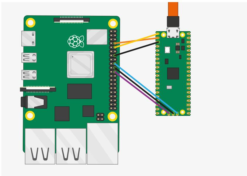
The default configuration is to have SWDIO on Pi GPIO 24, and SWCLK on GPIO 25 – and can be wired to a Raspberry Pi
