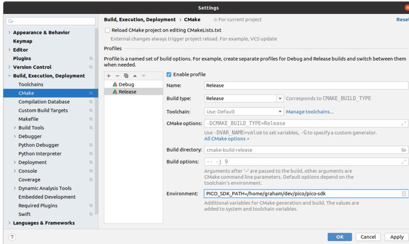
After pressing OK, you'll see something like Figure 34. Note that there are two tabs for the two profiles (**Debug** and **Release**) at the bottom of the window. In this case **Release** is selected, and you can see that the CMake setup was successful.
