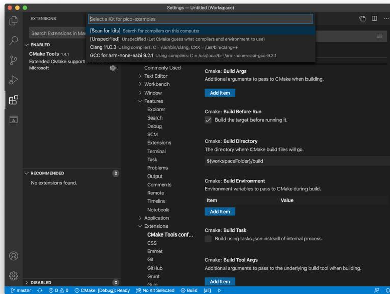
Finally go ahead and click on the "Build" button (with a cog wheel) in the blue bottom bar of the window. This will create the build directory and run CMake as we did by hand in [Section 3.1](#), before starting the build itself, see [Figure 9](#).
