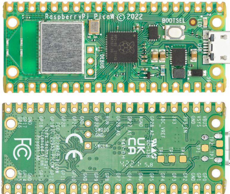
Raspberry Pi Pico W has been designed to be a low cost yet flexible development platform for RP2040, with the addition of a 2.4GHz wireless interface and the following key features:
