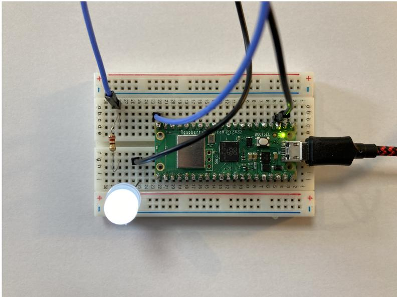
Connecting an LED to GP15 we can turn the LED on and off by using HTTP GET. We can do this by going to <http://192.168.1.X/light/on> to turn the LED on, and <http://192.168.1.X/light/off> to turn the LED off, in our web browser; where **192.168.1.X** is the IP address of our Pico W, which will be printed in the console after it connects to the network.
