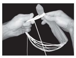
12. Attach the parachute to the shock cord at a point about 1/3 of the length of the shock cord from the nose cone. To do this, take the chute shroud line loop ends in one hand and, with the other hand, take the chute and go around the shock cord, passing the chute through the shroud
