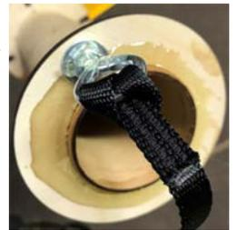
**STEP 4** Attach shock cord to FWD eye bolt. Pass loop through eye bolt, then pass shock cord through it's own loop as shown. This can be done prior to mounting motor tube assembly or fin can into airframe. Don't get any epoxy on the shock cord!
