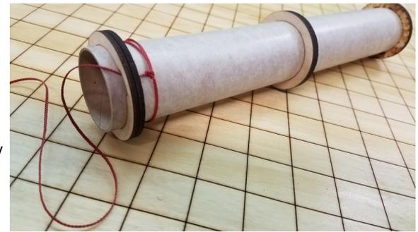
1. Take the length of 2' Kevlar cord and at its center make a 1" long loop knot and pull it tight. Make a knot a 1/4" away from the end of EACH of the two loose ends.
