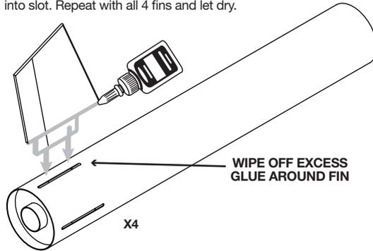
2. Apply glue fillets to all fin joints and smooth with finger.
