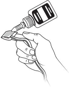
4. Glue shock cord to inside of body tube. Use finger to hold in place until glue sets.
