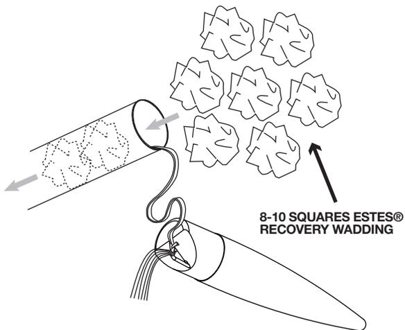
2. Fold parachute as shown. Wrap parachute lines loosely and insert into body tube. Recovery wadding and parachute must slide easily into body tube; redo if too tight.
