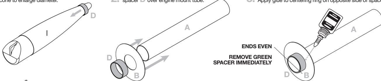
4. Slide centering ring C and green spacer over engine mount tube as shown.
