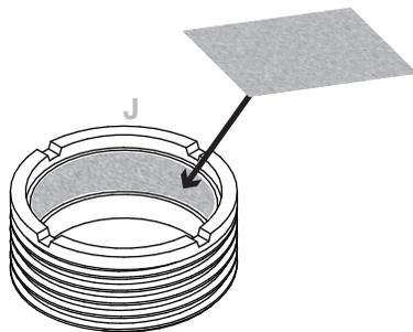
2. Attach with epoxy. Mix and apply according to instructions.
