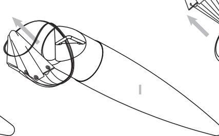
3. Tie shock cord to nose cone eyelet.
