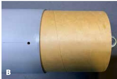
**B.** Next drill a 1/8" or 5/32" hole near the base of the payload section tube completely through the coupler. This hole is needed for high speed, high altitude flights to bleed off internal air pressure.
