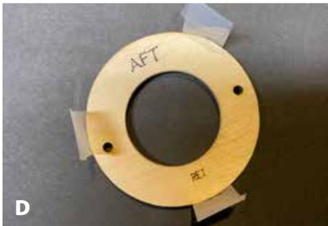
**D.** Make three or four cellophane tape tabs and apply to the AFT centering ring as shown above to aid in removing this ring at a later step.
