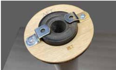
Loc has sold hundreds of kits using the standard Loc motor retainer system. Composed of two L brackets, bolts and retainer nuts, it's a simple but effective method of motor retention. This method is included with your kit. Using this method, the AFT centering ring mounts flush to the AFT end of the motor tube.
