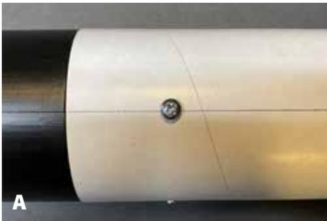
**A.** Slip the nosecone into the top of the payload section tube. Secure the nosecone to the payload section with small screws or removable plastic rivets equally spaced around the circumference of the payload section tube about 1" below the nosecone. Be sure to pre-drill holes of the appropriate size when using screws. 1/4" long sheet metal screws work well in this application. If you prefer to use PML Removable Plastic Rivets (RVT-24), you will need to drill 5/32" diameter holes.
