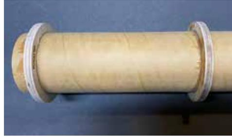
**B.** Dry fit all centering rings into the airframe and over the motor mount tube. The FWD and MID centering rings can be a little snug in the airframe and on the motor tube. If it is too tight, sand the ID and/or OD for a better fit.
