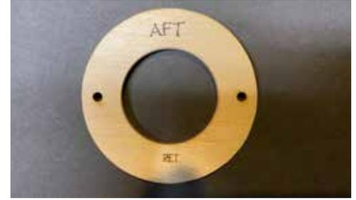
**C.** Use a pencil to mark the AFT centering ring for identification. *You do not want to switch the MID and AFT centering rings during assembly!* The AFT standard centering ring should be looser in the airframe and over the motor mount tube; you will need to slip the AFT centering off the motor tube while it is in the airframe during a later step. Sand the ID and/or OD for a loose fit if necessary.
