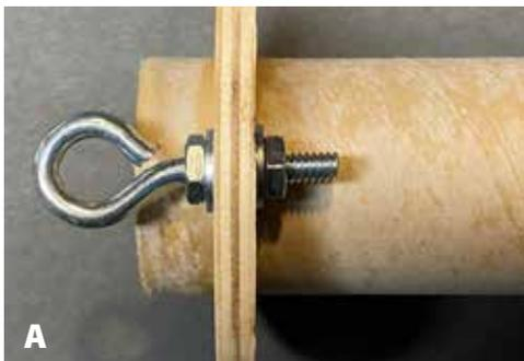
**A.** Install the eye bolt for the nylon tether. The eye faces forward; use a nut/washer/ centering ring/washer/nut. Tighten the nut securely. Make sure the eye does not interfere with the airframe - test fit!
