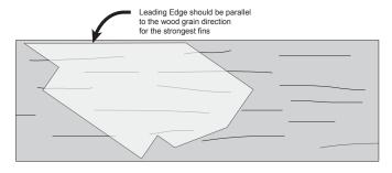
If your pattern is too big for a single sheet of wood, you can splice two pieces together using wood glue. Again, make sure the wood grain direction is parallel to the leading edge of the fin.
