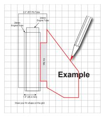
Photocopy your pattern 3-times. Cut out the pattern with a scissors. Put a low-tack adhesive on the back side (like Spray-Mount or rubber cement).
