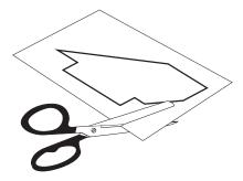
Place pattern sheet on your wood sheet. For the strongest fins, align the leading edge of the fin with the wood grain direction. Cut out the fins with a sharp hobby knife. Use a ruler's edge to help guide the knife when you make straight cuts. Peel off the paper pattern after the fin has been cut out.
