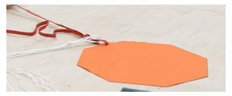
This knot should **not** be in the middle. The parachute should be attached closer to the nosecone- if both lines are pulled tight (like in freefall) the nosecone and airframe should not hit each other).
