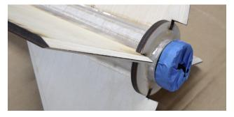
Tip: Wiggle the motor retainer as you slide it onto the motor tube to further disperse epoxy into those ridges.
