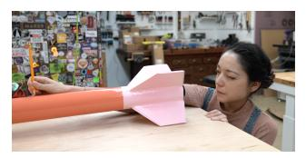
Eyeball the two points to be centered down the centerline of the rocket, between two fins. I've tried several ways of measuring this and honestly- eyeballing it seems to work the best. Just take your time and close one eye; you'd be surprised how accurate the human eye can be!
