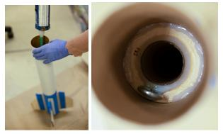
Before the epoxy cures, carefully peel up the masking tape to reveal a clean filleted edge that will need minimal sanding once the epoxy has completed setting.
