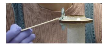
Use a gloved finger to clean up any epoxy that may have squeezed into the inside of the motor tube.
