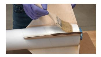
Carefully lay the fiberglass down and press it flat so it conforms to all the curves and surfaces. I find it easiest to start in the middle and work your way out to the fins.
