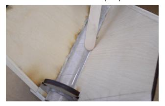
Before this epoxy cures, also use the Thixo epoxy to glue the aluminum motor retainer to the bottom of the motor tube. Be sure the threads of the motor retainer are masked off so you don't get epoxy in them.
