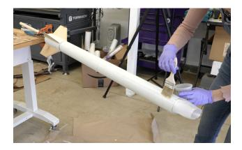
TIP: the cut edge of the fiberglass will fray and cause problems. That is a normal albeit frustrating part of the process. Refrain from pulling at the loose strands- it is better to cut them off if needed. (Your scissors can be washed with acetone to remove wet epoxy when you're done.) The best way to deal with this is to finish wetting out the rest of glass before getting to that edge, and then use a stippling motion on the raw edge instead of a brushing motion with your chip brush.
