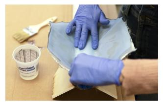
Be sure to smooth the surface of the peel-ply and gently squish all the bubbles out. The surface of your peel ply will be the surface of your epoxy, so the smoother you get it the less sanding you'll have to do!
