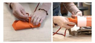
Load the burrito into the rocket- slide it to the bottom. We want it to protect the recovery line as much as possible too.
