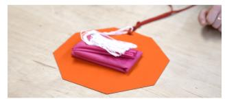
Wrap the parachute into the fire-resistant nomex like a burrito. It is important to protect the parachute and lines from the black powder ejection charge that will blast the nosecone off and parachute out.
