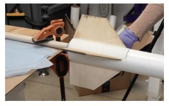
Mix up a larger quantity of **TotalBoat High Performance 2:1 epoxy** and paint a thin layer of epoxy on the tube all the way around.
