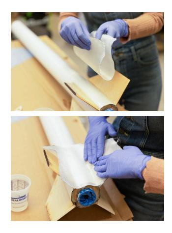
Slowly wet out the fiberglass with a brush, don't go too thick anywhere or the fiberglass will start bubbling and shifting around.
