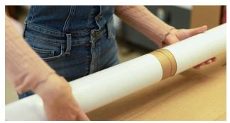
TIP: It is perfectly reasonable to separate at this joint as a payload section instead of deploying the nosecone at apogee. I do not recommend for beginner builders but if you need to fly your rocket in a suitcase to your launchsite this may be easier for transport, the instructions will not cover that though. **STEP 7:** Prep nosecone
