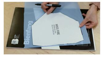
TIP: Sharpie bleeds through both fiberglass and peel ply so protect your table!
