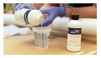
Mix up your **TotalBoat High Performance** epoxy and paint a thin coat of epoxy onto the fin area.
