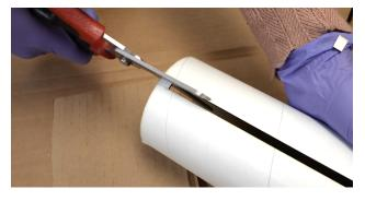
Before moving on to the next epoxy step, mask off the motor retainer to protect it while you're applying adhesive to the rest of the exterior of the rocket. (It may still be masked from the previous step)
