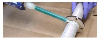
Once the centering ring is placed and secured with the adhesive, you're ready to glue the fins in place. Run a generous bead of epoxy down your marked lines. Firmly press the fin into place– squeeze out is a good sign.
