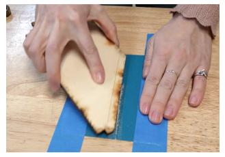
When working with epoxy, and any adhesive really, sanding laser cut edges thoroughly ensures better bond surfaces.
