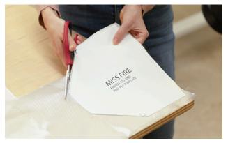
Trace that shape onto the fiberglass 4x and cut it out, then trace that shape onto the peel ply 4x and cut it out.
