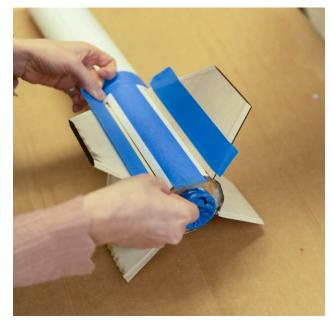
Run a bead of Epoxy around each of the fins, and before moving on to the next fin, use the rounded end of a popsicle stick to smooth those into a nice radius - using any excess to fill gaps.
