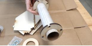
Note: the bottom edge of the fins should line up with the bottom of the motor tube.
