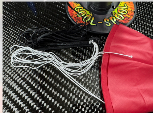
Slide fire blanket onto shock cord. Attach recovery. Add decal to top plate. Add decal to body tube.
