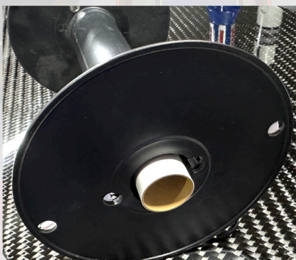
Insert assembly from top. Align launch lug holes. Glue top plate in place.
