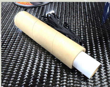
Sand centering rings to fit spacer tube. Motor tube should protrude from spacer tube. As well when test fit, protrude from base for motor retention. Glue motor mount in spacer tube.
