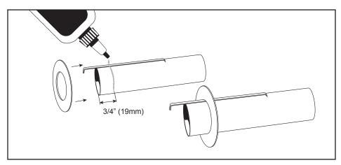
☐ 8. Remove a second engine mount centering ring from the die-cut card sheet. Apply a bead of wood glue around the front end of the engine mount tube. Slide the cardboard ring onto the engine tube near the front of the tube. Check to be sure the ring is aligned straight as shown.
