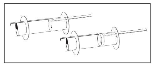
☐ 10. After the glue on the engine mount is dry, put a fillet of glue on each side of two the centering rings. These rings take a lot of stress at engine ejection, and you must make sure to have a good glue bond.
