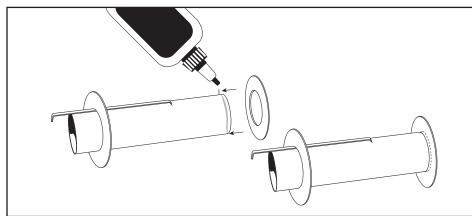
☐ 9. Engine block installation: Using wood glue, glue the green centering ring into the forward end of the engine mount tube. Push it in until it rests against the top of the engine hook. Once it is in place and dry, add a fillet of glue around the front edge of the green ring (engine block) using a long wood dowel.
