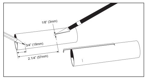
☐ 7. Remove one of the engine mount centering rings from the die-cut card sheet. Apply a bead of wood glue around the engine mount tube 3/4 inch (19mm) from the aft end. Slide one of the cardboard rings onto the engine tube over the engine hook and into the bead of glue. Check to be sure the ring is aligned straight, as shown. Allow the glue to dry.
