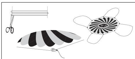
☐ 43. Holding the parachute at the center of its top, pull the lines together to even up the ends. Thread the 4 looped lines through the loop at the base of the nose cone. Take the top of the parachute and pull it through all 4 string loops at the same time and then pull to tighten the knot. This securely attaches the parachute to the rocket.
