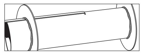
☐ 11. Cut out the "Stuffer-Tube" marking guide, P/N 37029 (B). Wrap the guide around the stuffer tube (AT 41.6/18) and tape the ends together. Mark a small line at each of the arrow points and label "top" and "bottom" as indicated on the marking guide, then remove it. Draw a pencil line down the entire length of the tube for both lines. Label one end of the tube as "front."
