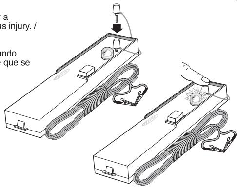
NOTE: Safety key is designed to remove itself when not held down. This breaks continuity to deactivate controller. /
