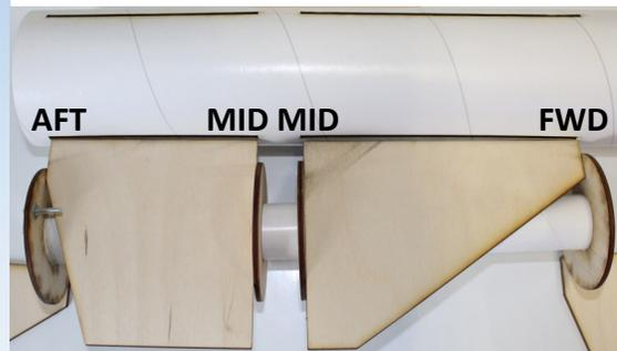
Good practice is to sandwich the fins between the rings. Align rings on motor tube as shown. Insert the fins between AFT/MID—MID/FWD rings to obtain proper alignment. Remove test fins. Ensure rings are perpendicular to the motor tubes and tack into place with epoxy. Once cured, make an epoxy fillet to the joint where the motor tubes
