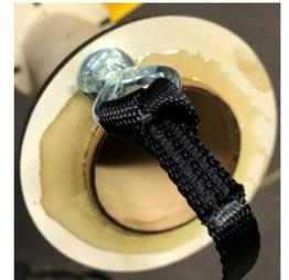
**STEP 3** Flip airframe over so AFT is upright. Apply an epoxy fillet to the intersection where the AFT ring meets the airframe. **DO NOT** get any epoxy in the motor tube or the T-nuts! Allow to cure.
