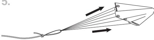
6. Attach shock cord to bottom of nose cone and tie double knot.
