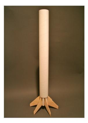
$\Box$  Make the main airframe tube with a line the entire length of the tube. Make the line on the main airframe tube 3" from the top of the tube.
