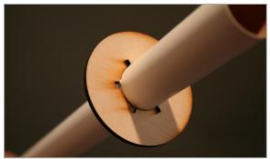
□ Using epoxy, glue the aft centering ring in place, taking care not to get any glue in the slots. After the epoxy has cured, trim away any excess adhesive in the slots.
