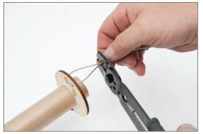
□ Place the other loop/sleeve connector on the free end of the cable. Make a 1-2" diameter loop and thread the free end back through the loop/sleeve connector. Crimp the loop/sleeve connector with a crimping tool or a pair of pliers. Apply a drop of CA to the joint.
