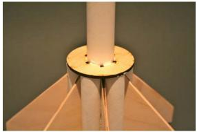
□ Locate the steel cable and the one of the loop/sleeve connectors. Thread one of the loop/sleeve connectors on to the cable. Then, thread the cable down through the top of one hole in the centering ring. Pull it back through the other hole and thread the end of the cable back through the loop/sleeve connector. Crimp the loop/sleeve connector with a crimping tool or a pair of pliers. Apply a drop of CA to the joint. Slide both of the heat shrink sections onto the cable.
