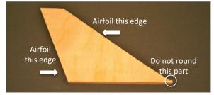
$\Box$  It is a good idea to sand and seal the fins prior to bonding it on the airframe. Cover the fin root with a strip of  $\frac{1}{2}$ " wide masking tape. The fins can best be sealed with finishing epoxy, balsa filler coat, or primer paint. Apply a coat of filler, sand smooth, and repeat the process until the wood grain is filled and the surfaces are smooth.
