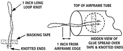
2. Cut a piece of masking tape 1/4" wide by 1 1/4" long. This is centered crosswise just ahead of the two knots.
