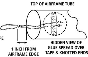
4. Place a generous bead of epoxy over the knotted ends and length of masking tape. Spread the epoxy around until they are completely covered and place the airframe in a horizontal position to dry.
