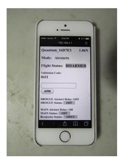
There are also a few differences. First, instead of display "DROGUE Time" and "MAIN Altitude", it displays "DROGUE Airstart Delay" and "MAIN Airstart Delay". There is no link next to these to change the values; they are all done from the Settings screen, since they are relatively complex. It also displays "Breakwire Status" (either OPEN or CLOSED), which is the current status of the breakwire input (more on that later).
