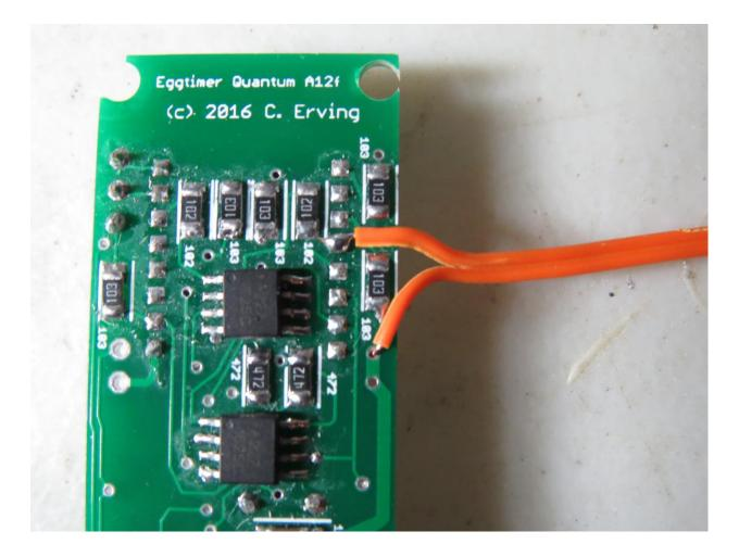
Note that this picture is of an early Rev A12f Quantum; the newer versions have a dedicated BW and 3V3 pads, so you don't have to tack-solder wires to the WiFi module.
